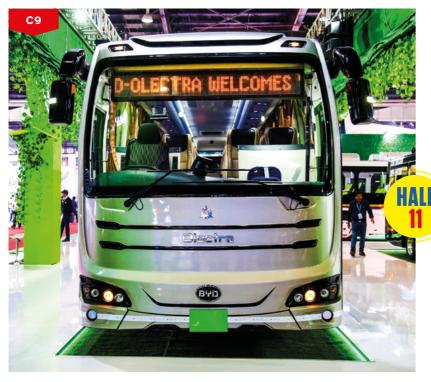
ITIN GADKARI, UNION Minister for Road Transport & Highways, Shipping and MSME, unveiled Olectra-BYD's C9. India's first electric inter-city coach. The long-distance Intercity Electric Bus gets a seating capacity of between 45-49 depending on the configuration. The 12-metre C9 can travel up to 300km in a single charge with a lithium-ion phosphate battery with fast charging capability, allowing it to be fully charged within three hours.
