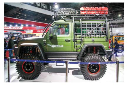
POWER IS TRANSFERRED TO ALL THE FOUR WHEELS VIA UNIMOG SOURCED PORTAL AXLES that the lockers on the portal axles can be engaged and disengaged on the fly. The suspension is upgraded with a lifted independent multi-link suspension all around. Both the front and rear share a similar setup - dual Bilstein hydraulic coil-over shock absorbers with dual-coil springs, one out of two shocks on either side. The maximum suspension travel is 300mm on both ends.
