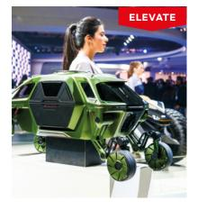
Hyundai claims it can traverse terrains beyond the reach of even the most capable off-road vehicle, courtesv a combination of a robotic leg architecture with wheel-hub propulsion motors allowing it to both scale obstacles such as a five-foot wall, as well as extend its 'gait' (over a five-foot gap, as claimed). It is unlikely the Kite or the Elevate will make it to production, however they do give us a fresh new perspective on what the future of mobility could be like.
