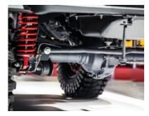
under the hood. The engine is in the same tune as in the standard Gurkha. It makes 88bhp and is mated to the same 5-speed manual gearbox with transfer case. The power is transferred to all the four wheels via Mercedes-Benz Unimog' sourced live-portal axles with mechanical lockers. The custom rig is fitted with massive off-road spec Maxxis Trepador tyres that are 363mm in width, fitted on 17-inch rims. While Force Motors have not revealed
